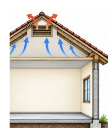
Attic heat ventilation
