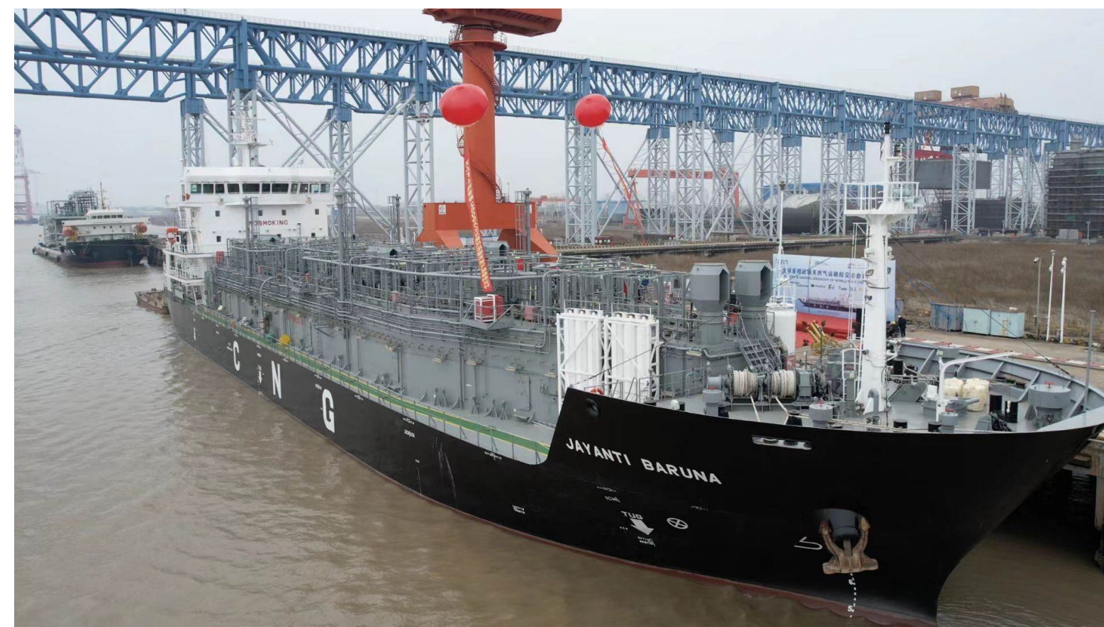
The Indonesian-flagged vessel owned by PT PLN is the world's first CNG carrier. The ship is also operated with dual fuel diesel
