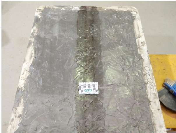
Sealed surface after wheel tracking
