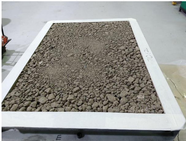
Surface after compaction
