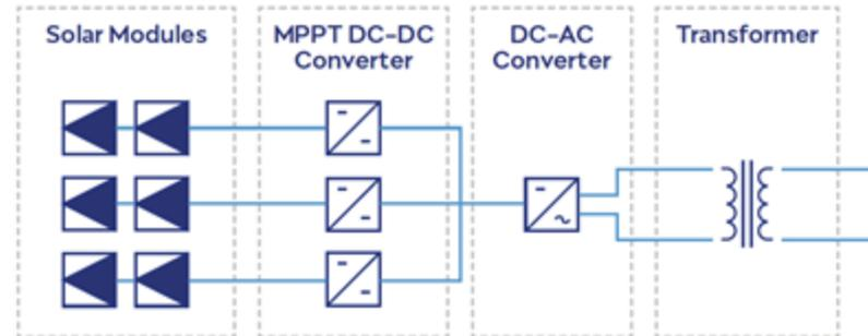
Fig 1. Daybreak converter development for connecting solar PV to 25 kV AC traction networks
