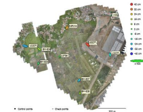
Fig. 5. GCP locations and error estimates. Z error is represented by ellipse color. XY errors are represented by ellipse shape. Estimated GCP locations are marked with a dot or crossing.
