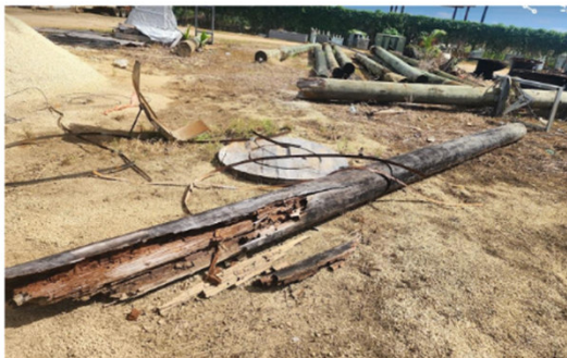
Figure 2 – Is a ATPFL pole at the TPL yard showing ground rot and decay from the base of the pole extending up to 3.0-4.0m.
