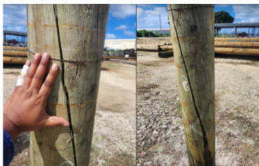
Figure 2 – Is a ATPFL pole at the TPL yard showing ground rot and decay from the base of the pole extending up to 3.0-4.0m.
