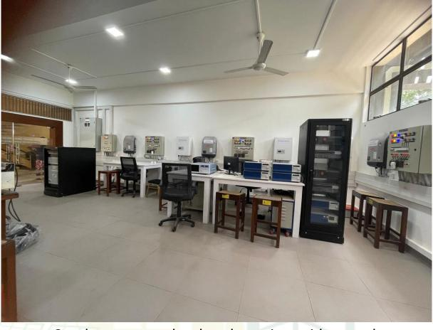
Conducts research related to microgrid control, power electronic control and optimization as well as real time simulation facilities
