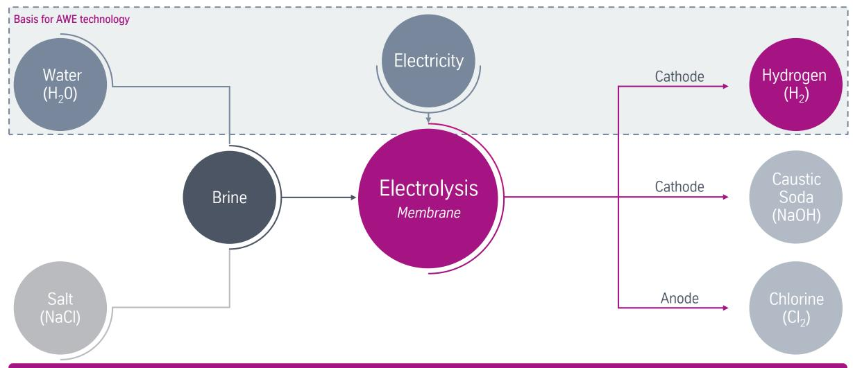
CA chemistry describes the process of splitting salt (NaCl) and water (H2O) into Chlorine (Cl2), Caustic Soda (NaOH) and Hydrogen (H2)
