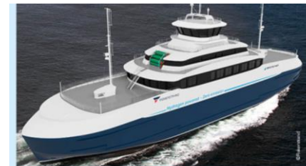
In the HYBRIDShip project of Fiskestrand Holding launched in 2016, a diesel-powered ferry was converted to hydrogen.
