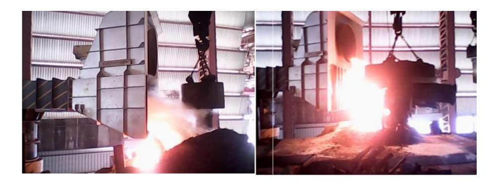
Sideways collection of fumes from melting and casting operation
