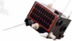
AIS, Digital & Video Cam, Amateur Emergency Comm Payload
