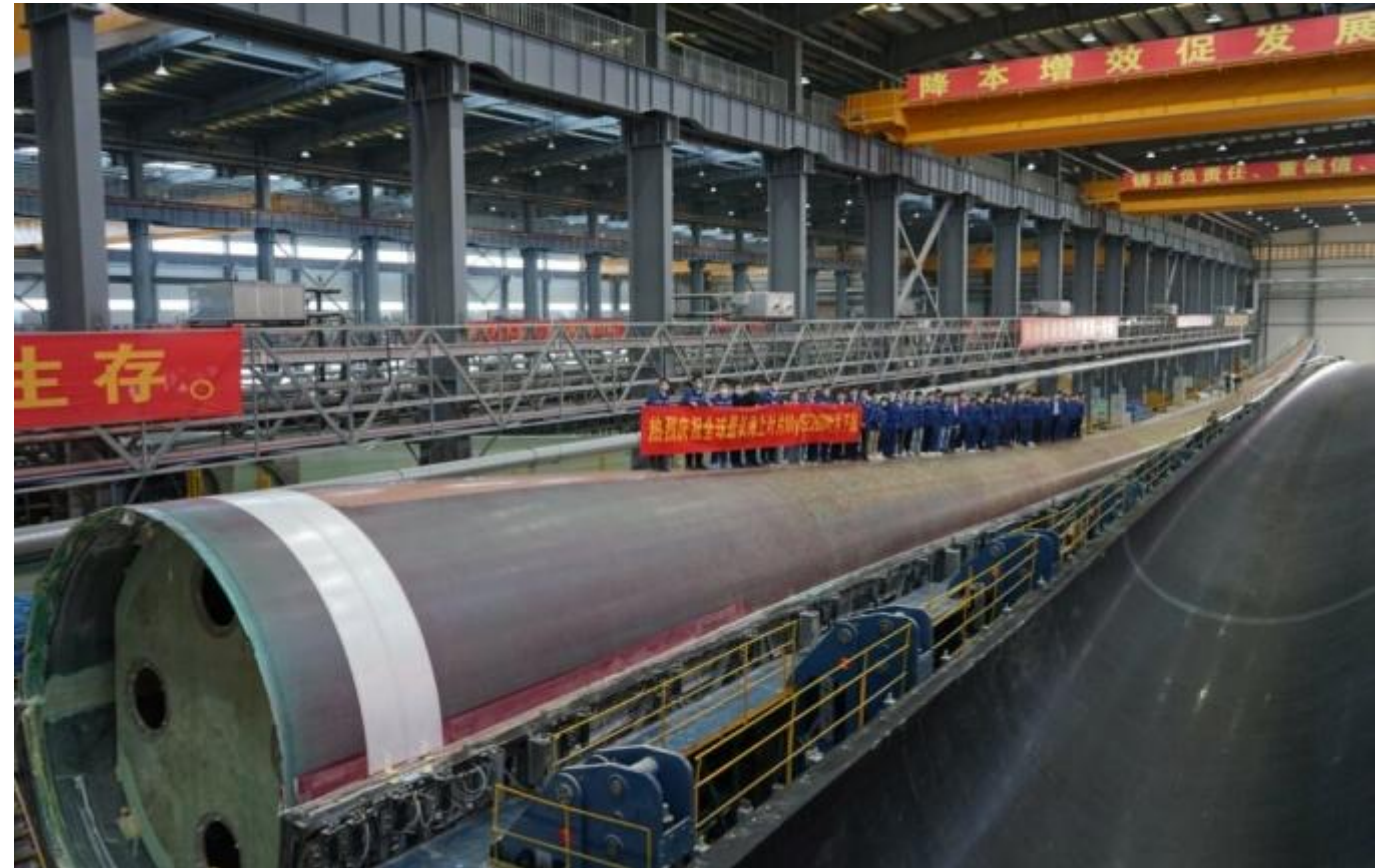
Mingyang Smart Energy 115.5 m long blade for 16.6 MW turbine with typhoon rating
