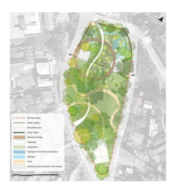
The Baguio City FEWS project's Flood Mitigation Action Plan includes a number of conceptual designs using nature-based solutions for existing places in the city.
