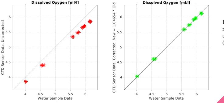
For this sensor type, recommended adjustment is gain only (no offset)
