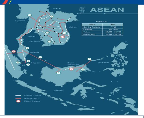
Realisation of ASEAN's cross-border interconnection system with higher penetration of variable renewable energy (solar and wind), under the ASEAN Power Grid.
