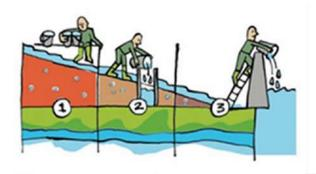
Three-step approach on drainage: retention, storage and drainage
