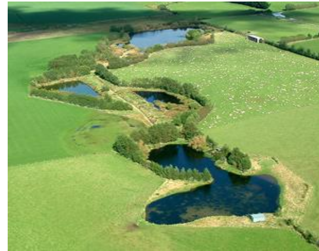
Integrated constructed wetlands (ICWs) for treatment of runoff from farmyards (Dunhill area, Ireland)
