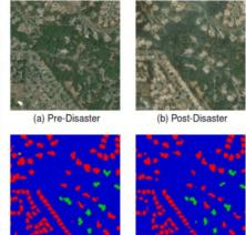
Fig. 1. Samples from the xBD dataset []] for building damage assessment. (a) and (b) respectively show Pre and Post Disaster images. (c) and shows ground ruth and prediction from proposed method. Red labels represent completely damaged buildings, and Green labels represent undamaged buildings. Intermediate damage levels are represented by pink (major damage) and orange (minor damage).
