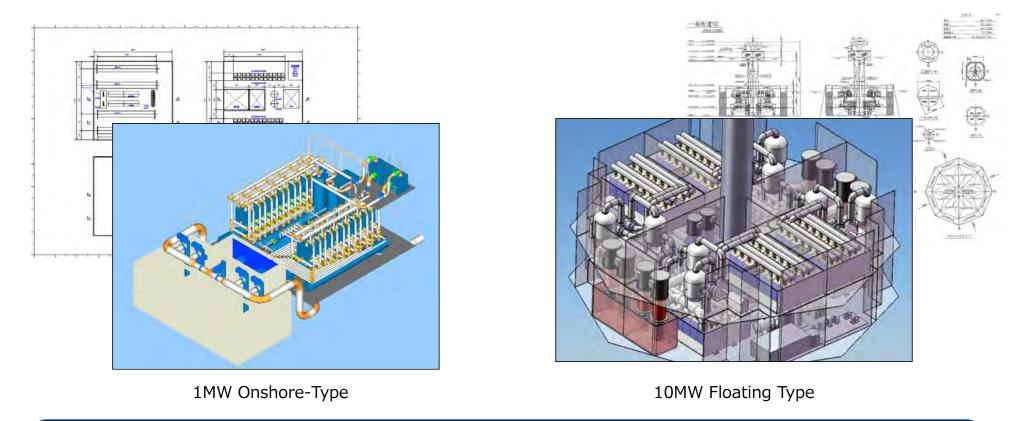
Binary Power generation systems are relatively simple, with few moving parts and no high temperature stress. Components are commercially available (more so at scales MW+). Preliminary design of 10MW floating plants have been completed in Japan.
