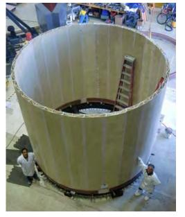
Prototype Composite pipe for 10MW OTEC
