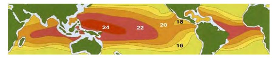
In the tropics and subtropics, there is a naturally occurring temperature difference between the surface ocean water (SOW) and deep ocean water (DOW).
