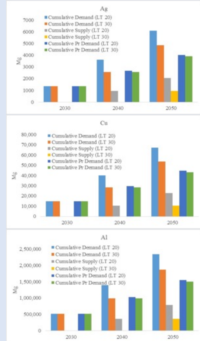
Cumulative demand and supply of materials in the PV solar technology in Qinghai
