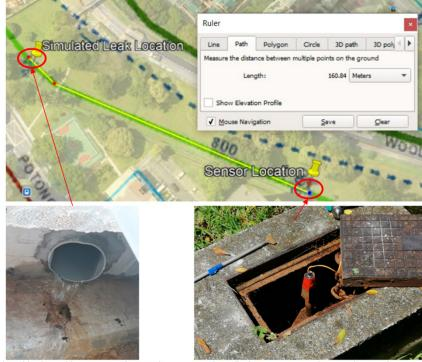
Simulated leak position at a washout valve
