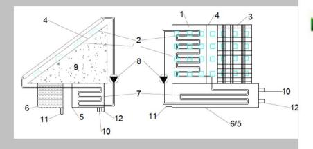
It is a combination of PV and thermal solar panels. Scalable, autonomous and mobile. SC evaporate dirty water. PV modules condensate clean water using TEM. The prototype is built. The patent is protected. Relevant for the regions without fresh water.
