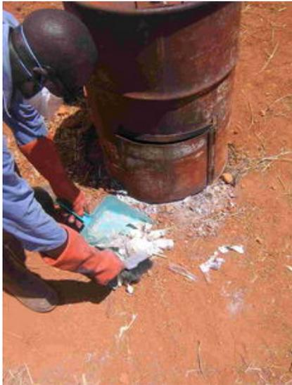
A person wearing a blue uniform and red gloves is using a blue dustpan to clean up white soft waste that has fallen on the ground around the base of the drum volume reducer. The drum is closed, and the person is focused on the task. |
