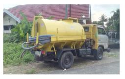
Figure 62: Desludging Equipment Operated by the Jambi Waste Hauler Companies
