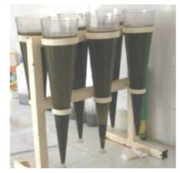
Figure 49: Imhoff Cones To Be Used for Determination of Sludge Volume Index
