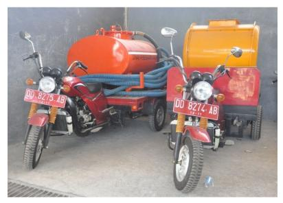
Figure 29: Vacutug-Type Desludging Vehicles for Septage Tanks with Difficult Access
