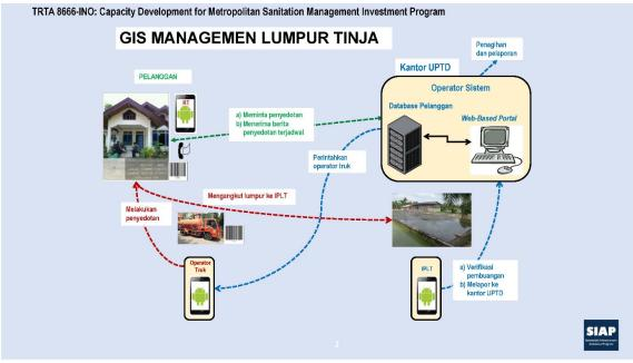
Figure 17: Data Flow and Desludging Truck Movement
