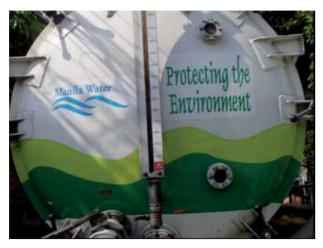
Figure 45: Calibrated Sight Gauge on Vacuum Truck to Estimate Tank Level<sup>46</sup>
