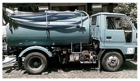
Figure 39: Vacuum Truck with Complete Equipment<sup>41</sup>
