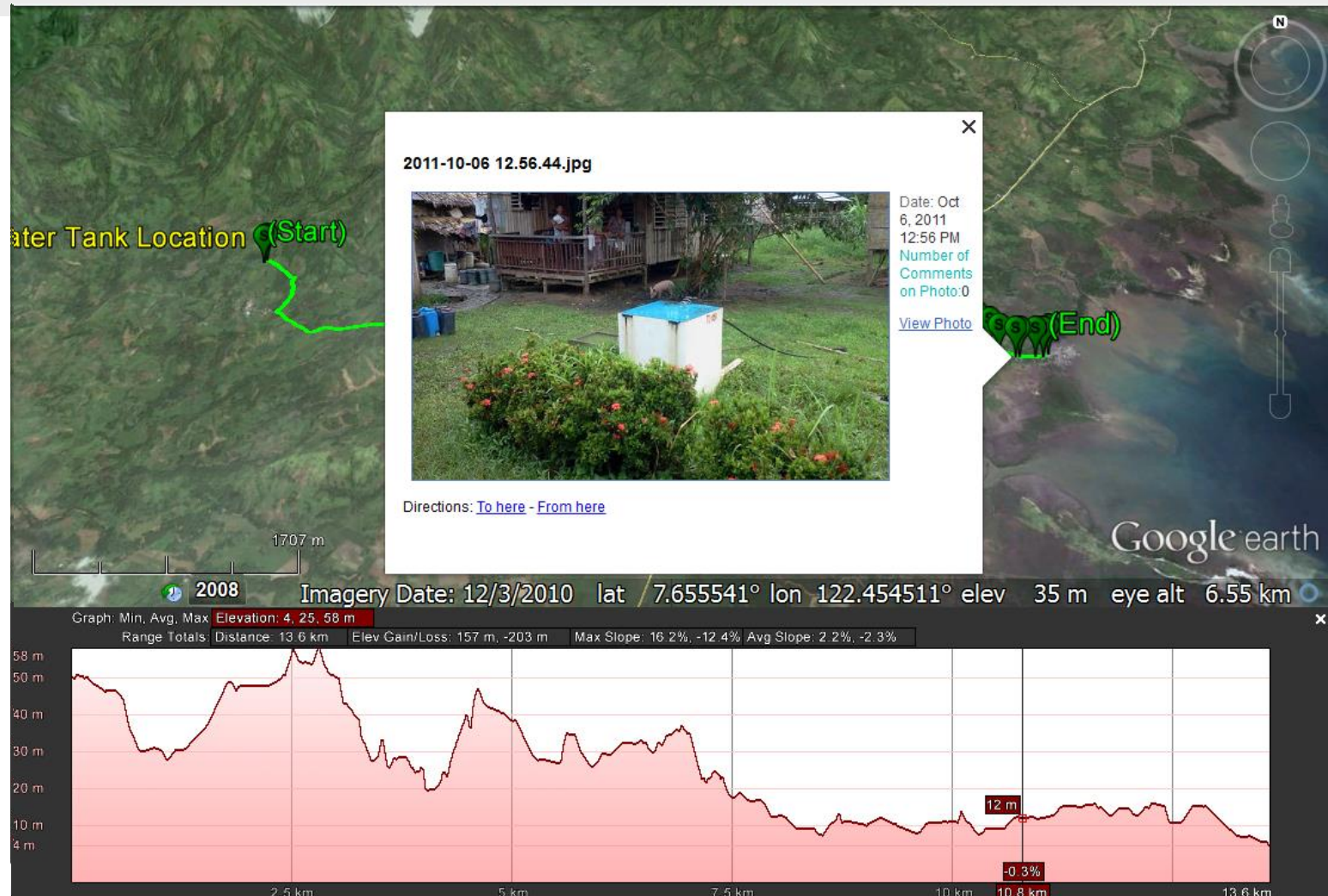
Geo-tagging Example No. 3 Visualization of a water supply project showing specific location, elevation profile from the source, distribution lines and faucets, and ground photos of community faucets
