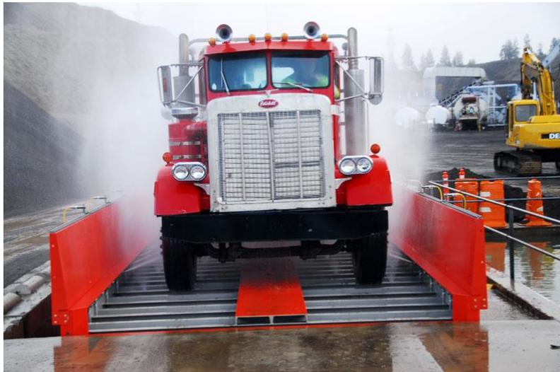
Access roads should be constructed from sandy/gravel material. If mud is noticed on the public roads near the entrance gate it must be immediately cleaned off by either water trucks and/or shovels. The wheel wash will require regular maintenance.
