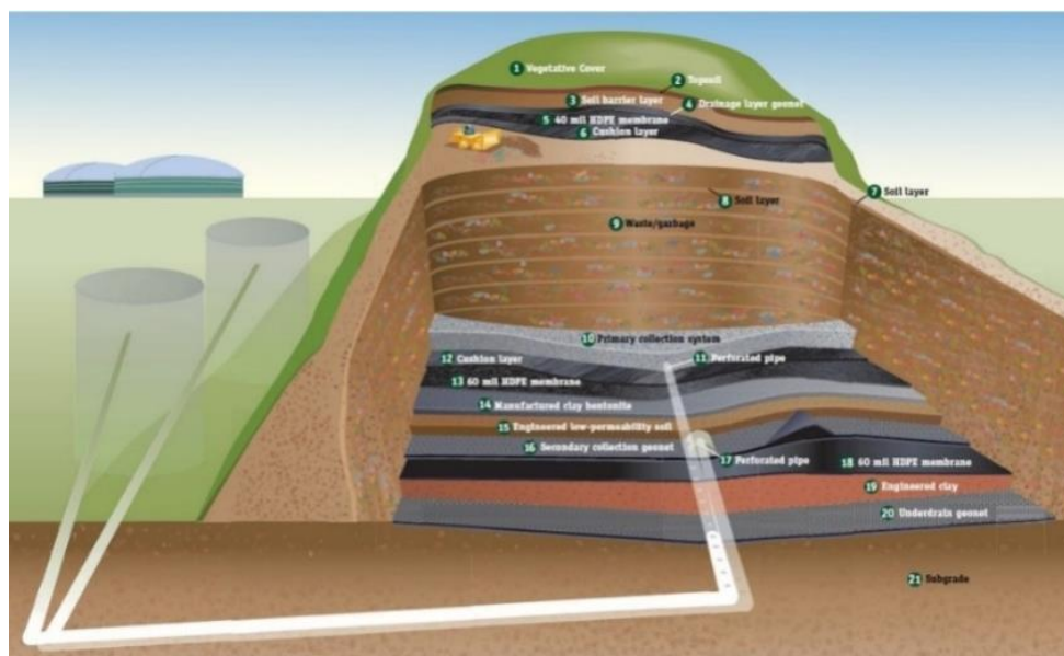
Figure 2-6: Schematic diagram of landfill site 11
