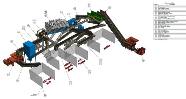
• Figure 3-3 Example of RDF Manufacturing Plant (3D model)
