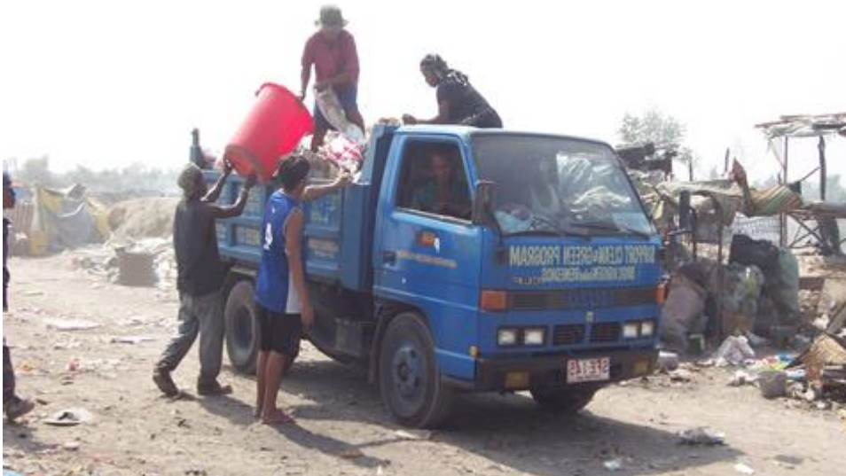
Collecting a waste sample from every truck load on the agreed audit days
