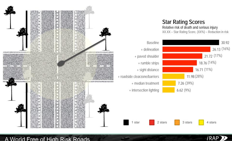
Level terrain, speed 80km/h, AADT = 10,000 vpd, 1 curve per km, 1 intersection per km
