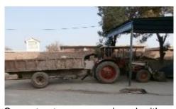
Some tractors are equipped with a front bucket that can lift the waste from the primary dumping locations into the trailer which is a significant labour saving benefit. Adding the loader element to the tractor adds more hydraulics and is now comparable to a skip bin truck excluding the body compaction elements.
