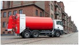
of a concrete agitator truck. Therefore the only moving parts are the roller bearings and one motor to drive the cylinder. When the waste has to be emptied from the cylinder, the motor is merely reversed and this spiral plate forces the waste from the vehicle. Such systems are becoming more popular throughout Europe and require far less maintenance than a typical waste compactor vehicles using the traditional ram system.
