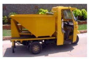
Therefore a number of the Riksaaf three wheel vehicles, or equivalent, capable of carrying 200 kg of waste could be utilised.
