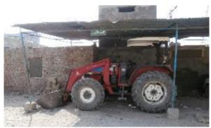
However the tractors are obviously slow when hauling to the landfill and even with the option of hauling more than one trailer, is still relatively inefficient. A hybrid combination could be to use the tractor-trailer for collection from the primary dumping locations hauling to a transfer station using large articulated tipper-trailers or 30m<sup>3</sup> hook lift bins.
