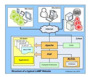
Figure 6-3: Illustration of Principal Component in the Architecture of a Typical LAMP Web Server
