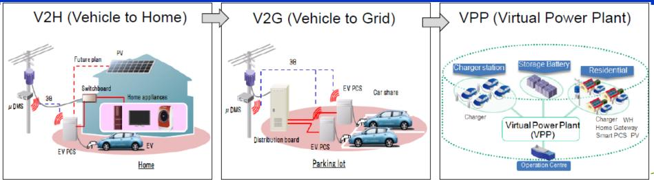
Virtual Power Plant (VPP): Aggregating and optimizing available distributed energy resources such as EV, storage and home side energy capability to use optional energy sources
