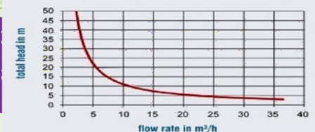
performances of "Sunpulse Water" at 300 W hydraulic power
