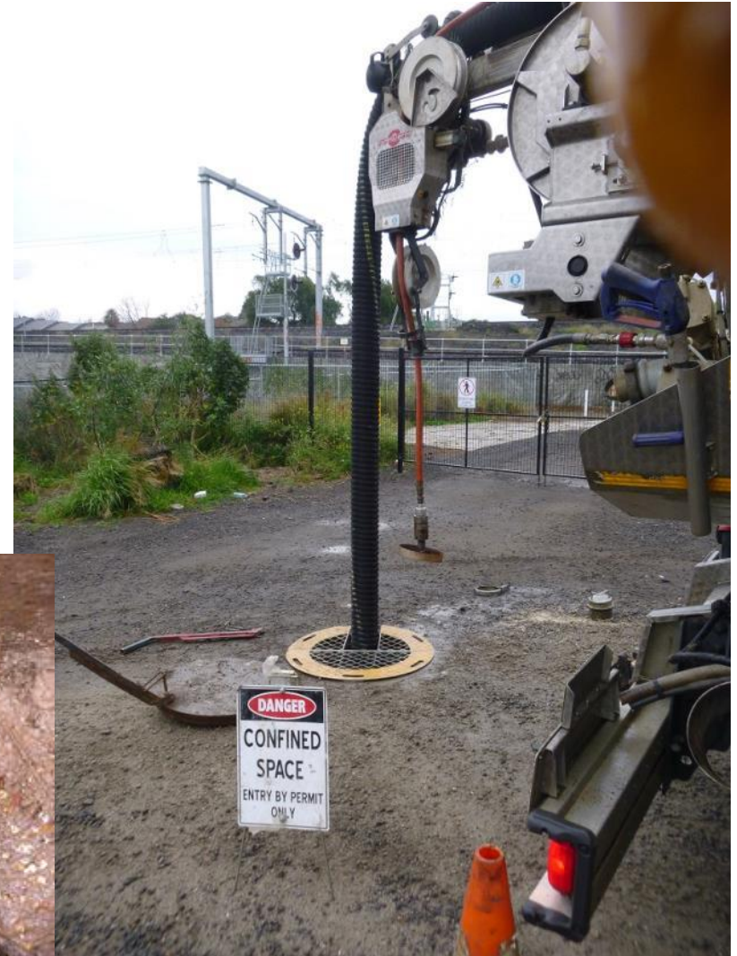
Combination Hydrovac Vehicle for Education, root cutting and jetting
