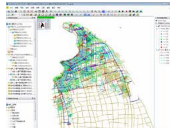
View of hydraulic model for Pudong displaying pressure zones
