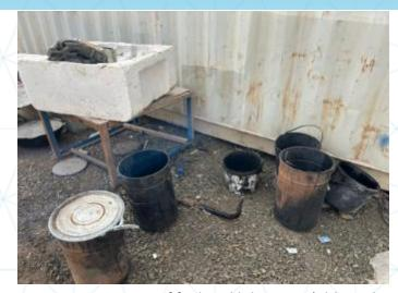
Improper storage of fuel and lubricants (old used barrels of fuel and lubricants)
