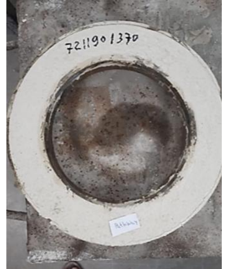
Pathway mix design – No cracks
