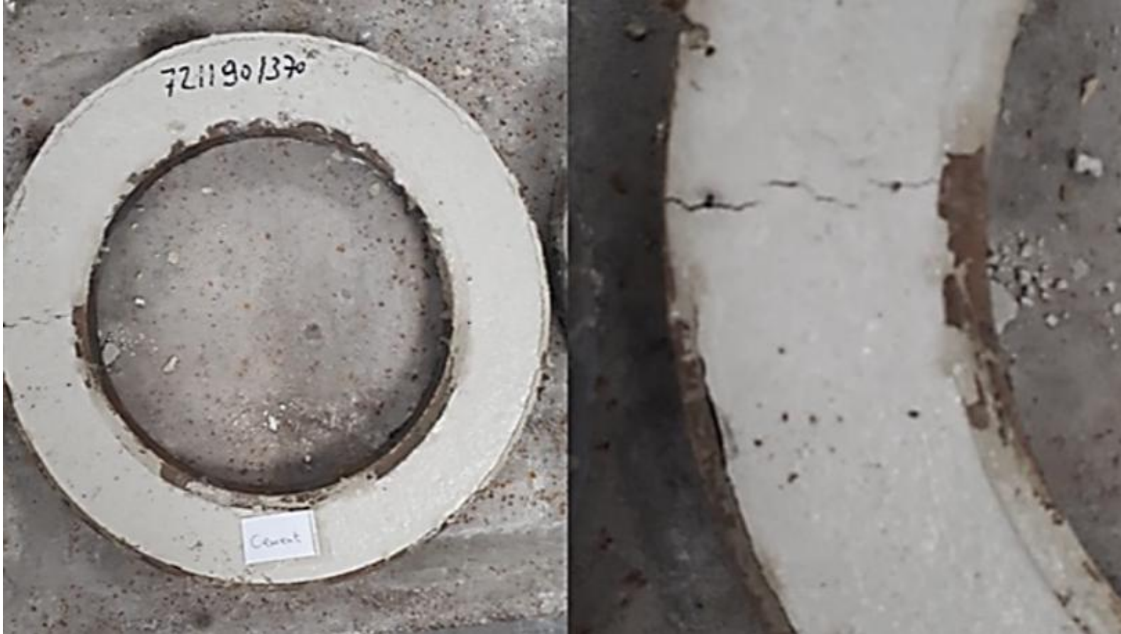
OPC with Pathway Aggregate developed cracks within 24 hours
