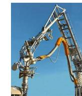
Liquefied Hydrogen Loading Arm
