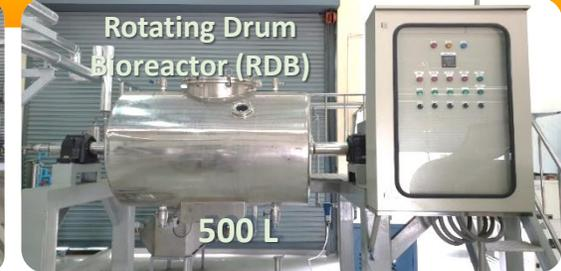
Rotating Drum Bioreactor (RDB)
