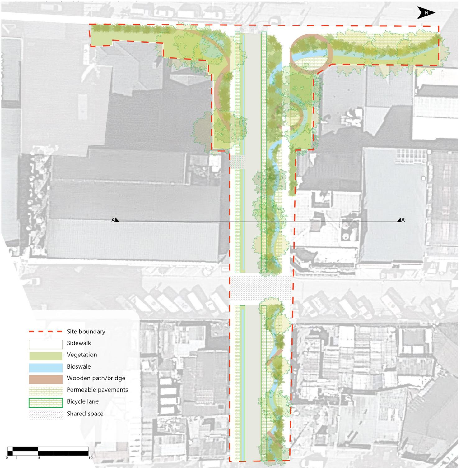
**Figure 23: Plan View of Green Street Conceptual Design at Carino St.**
