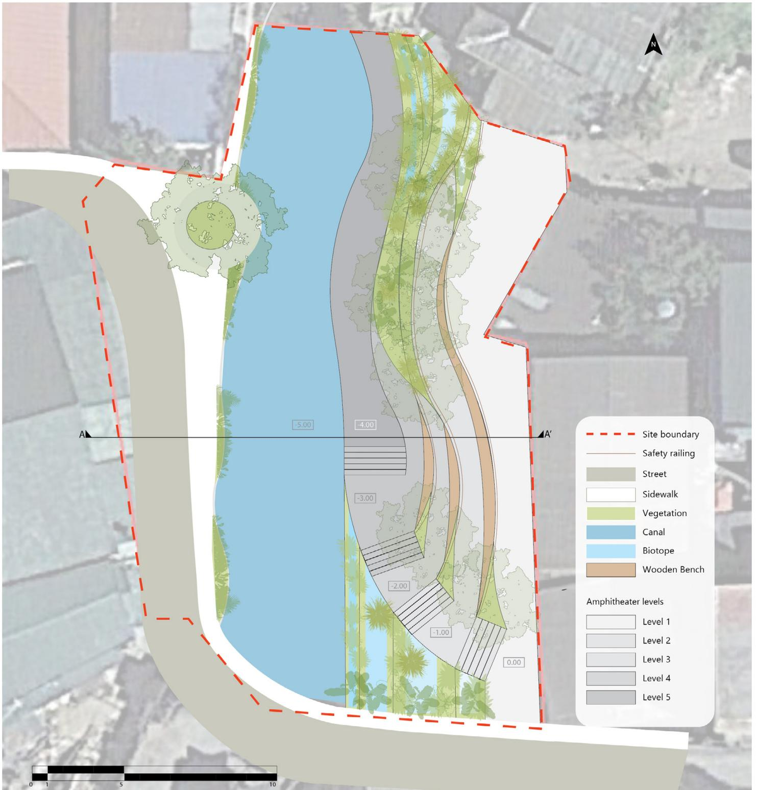
**Figure 21: Plan view of Urban Canal conceptual design**
