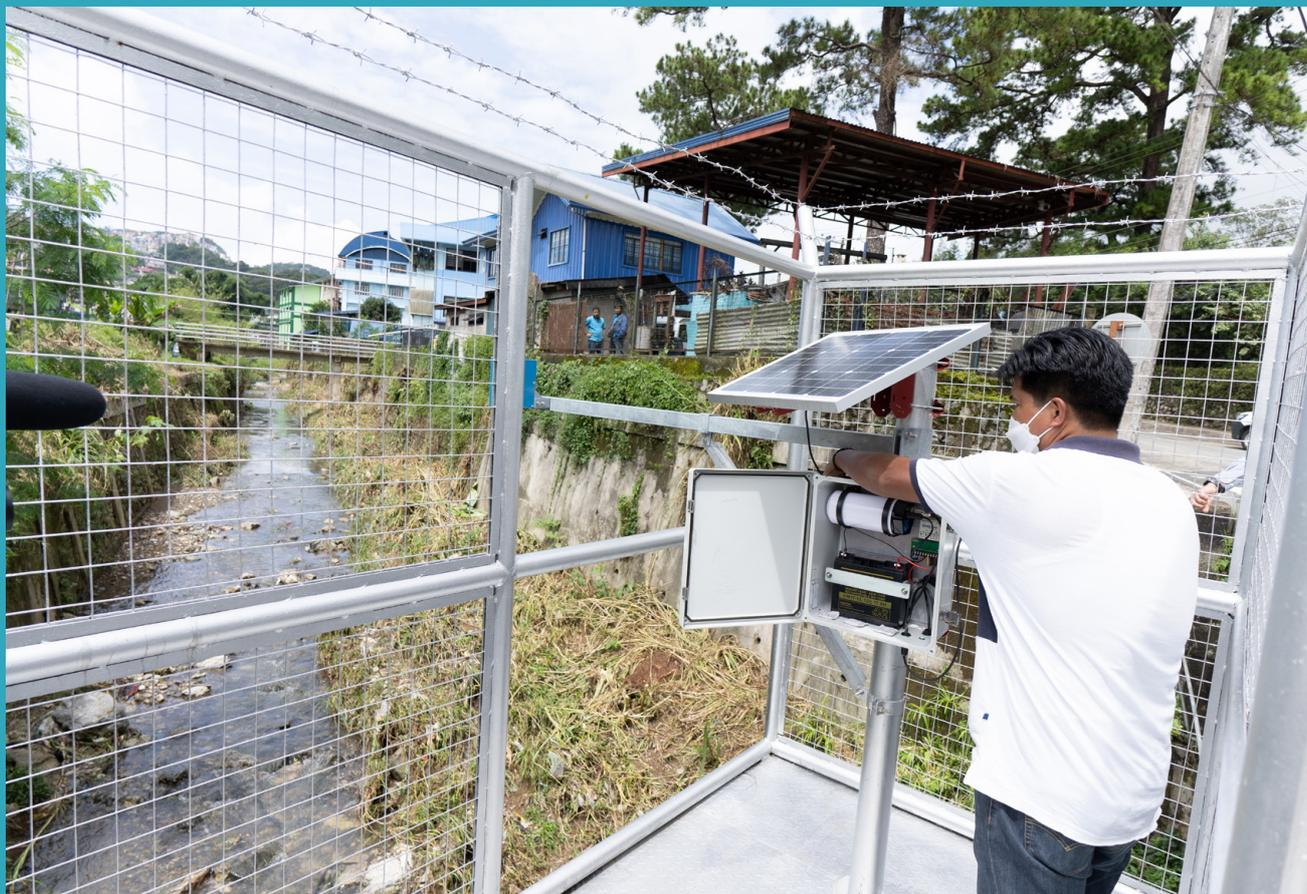
**Figure 40: Monitoring station at Fergusson Bridge. The station was constructed as part of the project in 2022.**
