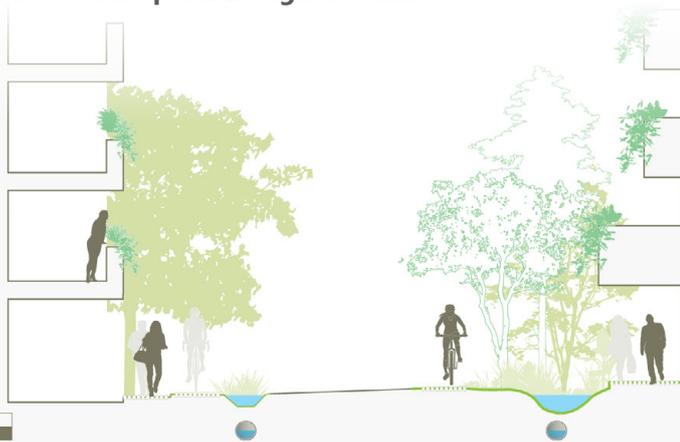
**Figure 24: Section AA' - Green Street Conceptual Design at Carino St.**
