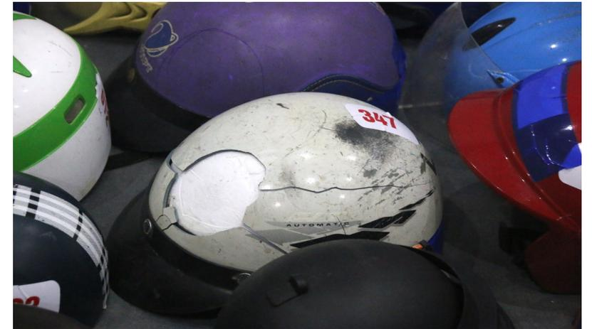
*A helmet breaks during weight testing.*
