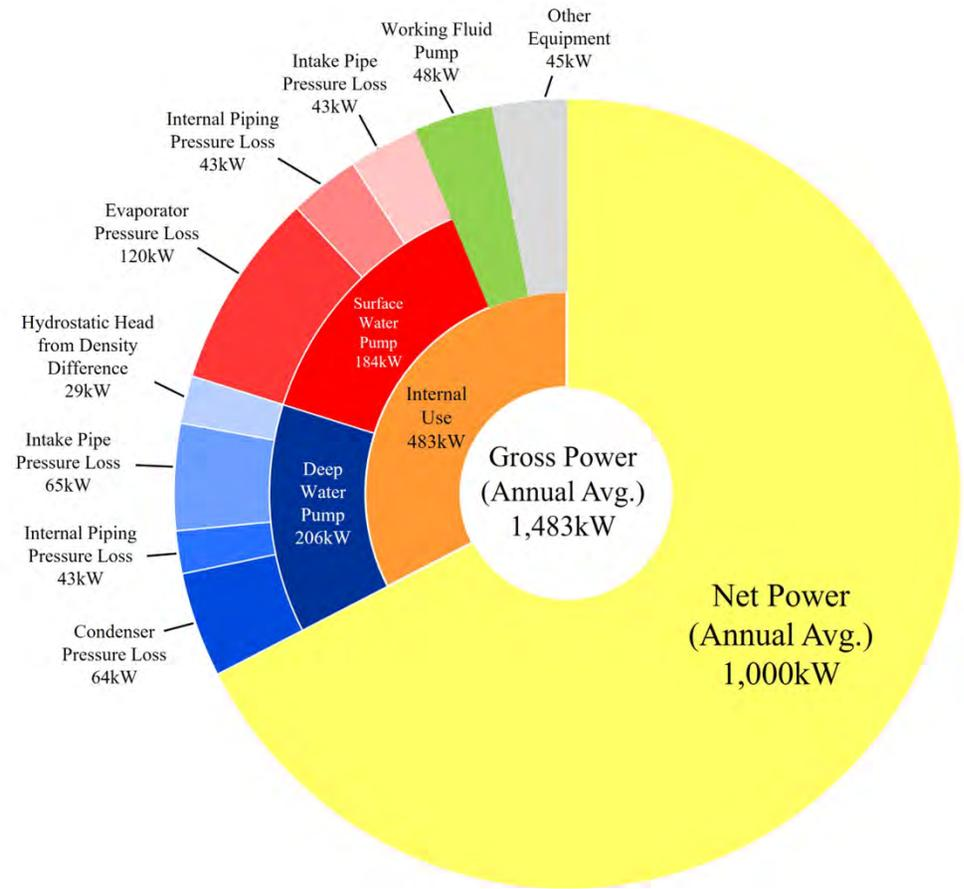
Breakdown of Internal Power Consumption for 1MW OTEC on Kumejima
