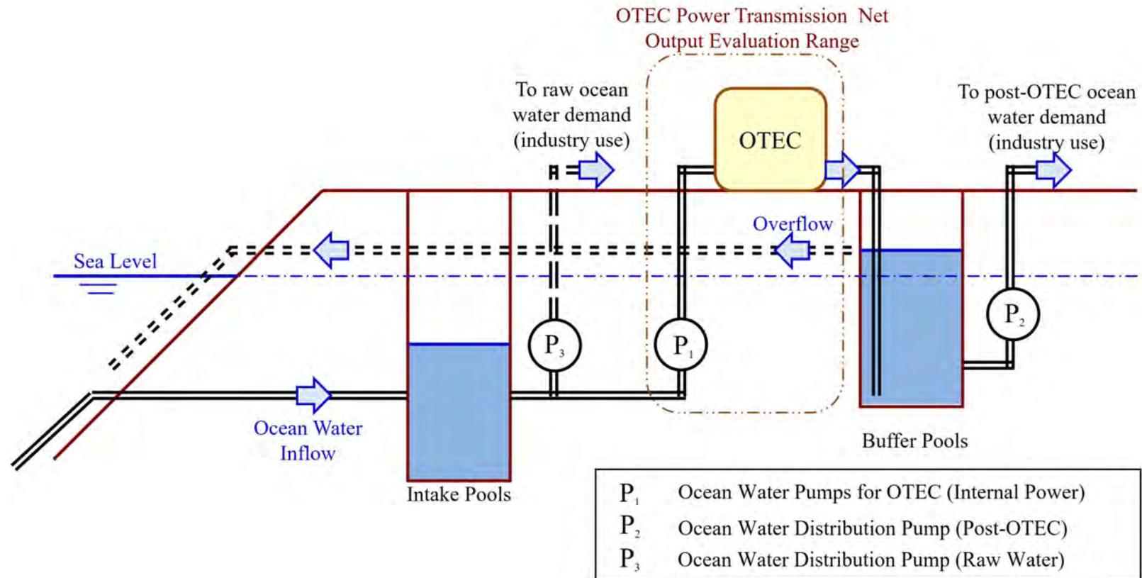
OTEC supplies varieties of water temperatures and clean energy for pumping and grid supply.
