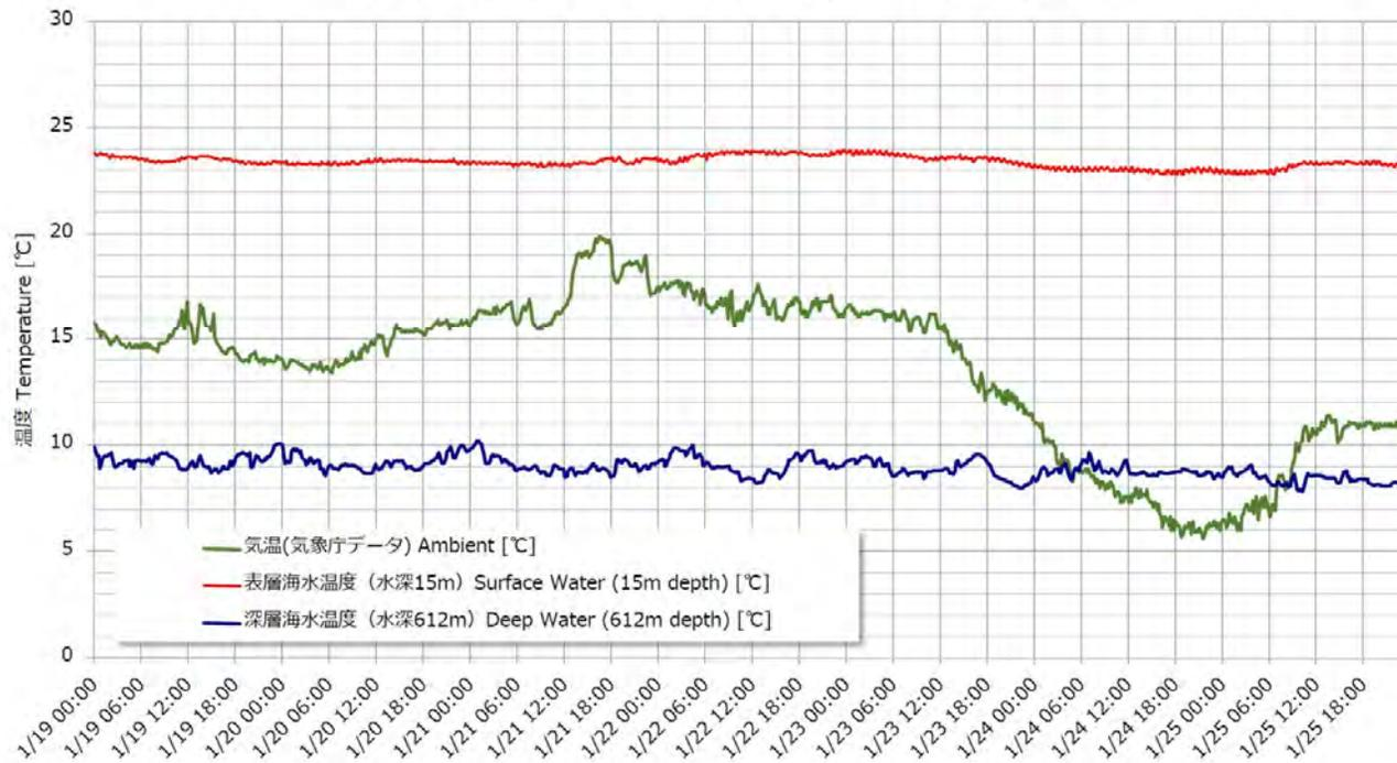
Ocean Water changes slowly compared to ambient temperatures, even during abnormal weather, as seen in the chart above. Combined with low fatigue, OTEC has a very **high capacity factor** (~90%) and stable output suitable for **baseload power**.
