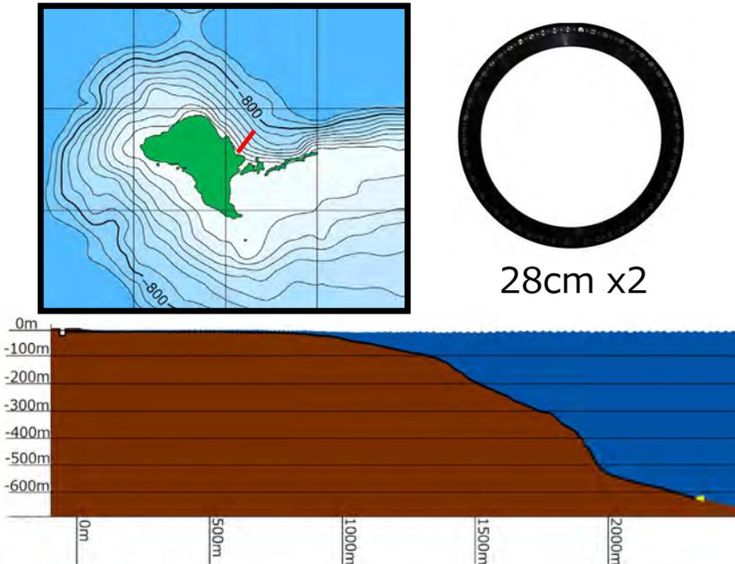
Onshore OTEC requires long intake pipes. Although initial cost is high, once installed they have very long operational lives and can contribute to various industry development.
