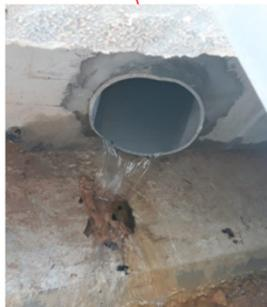
Simulated leak position at a washout valve
