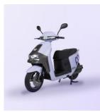
The e-Scooter connects two e-batteries in series, providing a high-performance driving experience with a motor power of 3 kW (50 to 80 cc).
