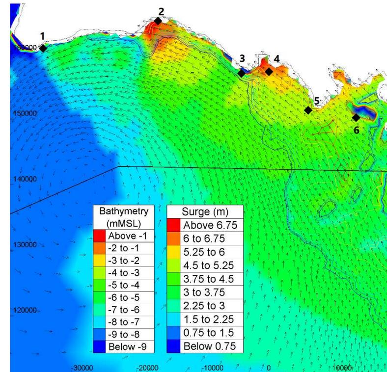
Maximum storm surge for event 004-00678-2 (coloured grid), TC track (black line), output locations (black diamonds), bathymetry contours (black line along the coast is the zero mMSL) contour and wind arrows
