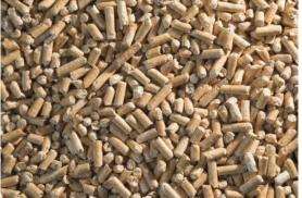
> Wood pellets produced by extruding dried, ground wood chips or other
