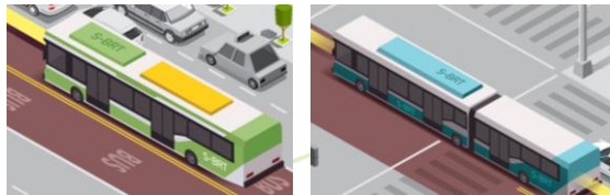
S-BUS (Articulated bus with doors on both sides)
