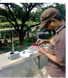
Installing and deploying Clarity Node-S to measure air quality in Bengaluru
