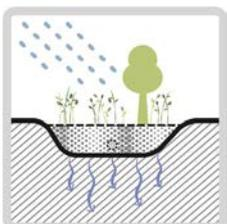
A gravel layer is a subsurface facility packed with gravel for infiltration of runoff. Runoff is carried above or below the surface and led into the layer or shaft. Such systems are used next to paved surfaces or next to unpaved surfaces that do not offer sufficient room for infiltration ditches or where the ground has an insufficient permeability factor.
