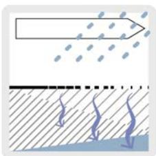
Amending soils improves the conductivity, or infiltration (in/hr) of the soil. This is achieved by increasing the permeability of the soil, allowing water to move through the spaces between soil particles more freely. Typically, native soils in the Greater New Orleans area consist primarily of compacted clays, which have small soil particles with little void space between. Replacing these clay soils with sandy soils, which exhibit large particles with a high void ratio, increases permeability.
