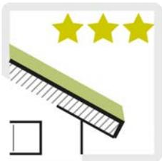
Intensive green roofs have a minimum depth of six (6) inches and are a layered system containing growing media, waterproofing membrane, drainage, and advanced irrigation components. Intensive green roofs can support groundcovers, bushes and even trees, and therefore require more structural support and maintenance when compared to extensive green roofs.
